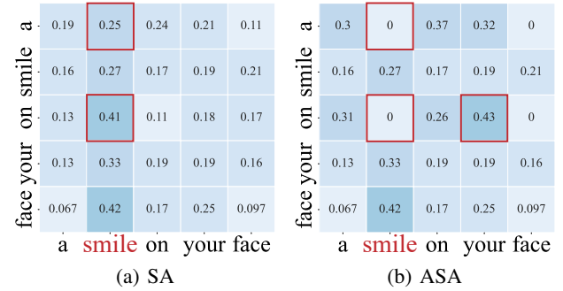
Figure 1: Empirical attention maps from SA and ASA of the first BERT layer. The text is a smile on your face from SST-2 dataset. The sum of horizontal scores is equal to 1. We highlight some units receiving strong attention diversions.
