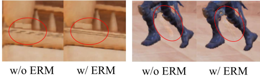
Figure 7: Effect of ERM. The module can recover the details in both the aliasing regions and warping holes.
