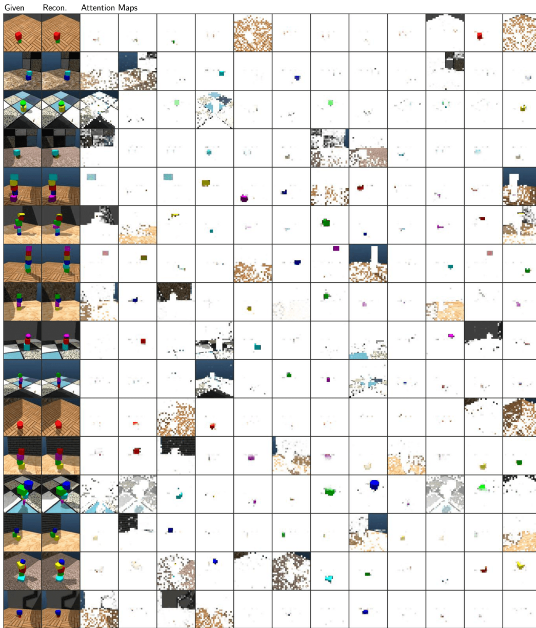
Figure 25: Reconstruction and attention maps of slots in SLATE given the input images for Shapestacks. We note that attention maps effectively localize on the individual blocks.
