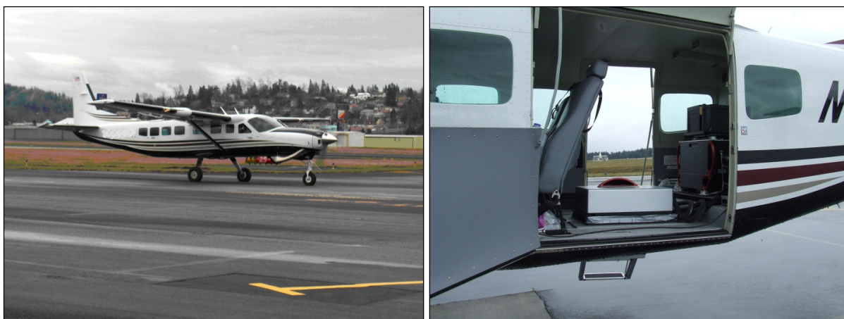
The Cessna Caravan is a powerful and stable platform, ideal for the terrain of the Pacific Northwest. The Leica ALS60 sensor head installed in the Caravan is shown on the right.
