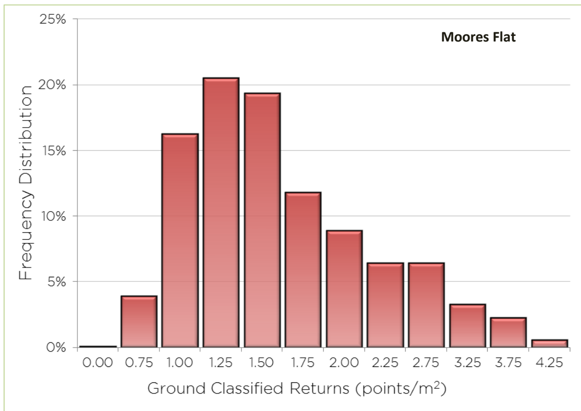
Frequency distribution of ground return densities of the 1m gridded study area for the Moores Flat AOI
