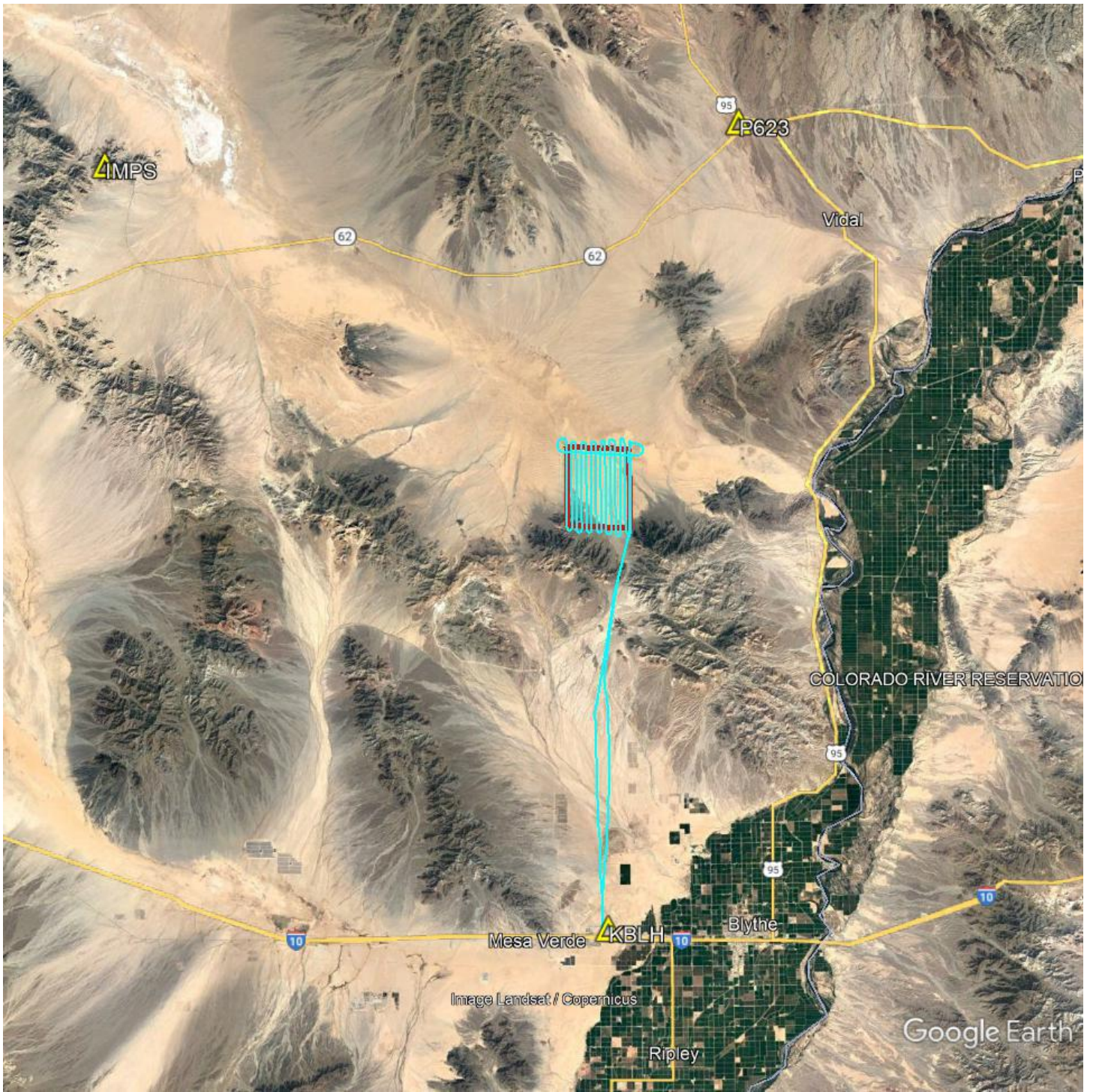
Location of survey polygon, aircraft trajectory, and GNSS reference stations
