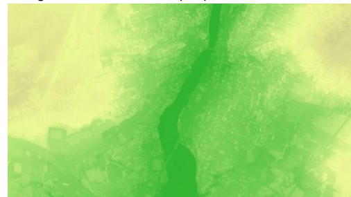
Figure 6: Color Relief Map representation of a DSM
