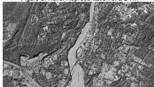
Figure 4: Relief Representation of a DSM
