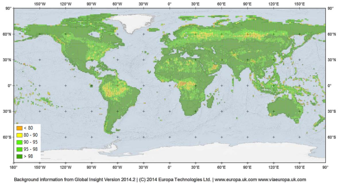
**Figure 17: Spatial distribution of relative, vertical accuracy statistics (LE90<sub>REL</sub>, from DLR, geotile basis, excl. Antarctica & Greenland)**
