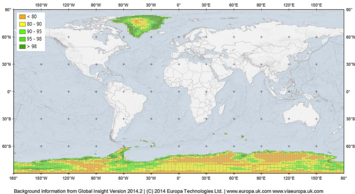
**Figure 18: Spatial distribution of relative, vertical accuracy statistics for areas with permanent snow/ice cover (Antarctica & Greenland, LE90<sub>REL</sub>, from DLR, geotile basis)**
