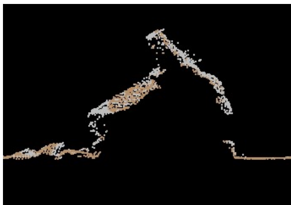
Figure 15: LAS point cloud profile view from previous – post editing - introduced ground points
