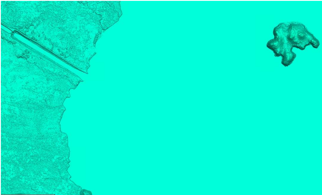
Figure 28: Example of a hydro-flattened DEM Lake Tile DEM_BH35_2021_1000_2611
