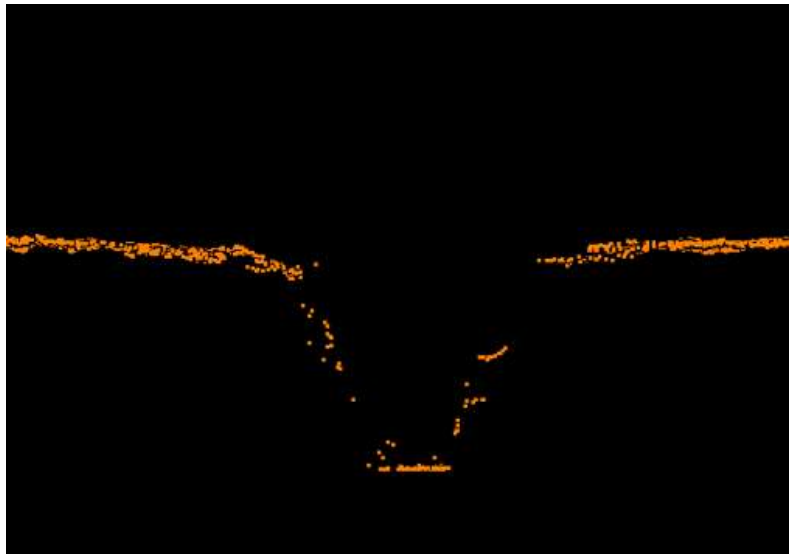
Figure 15: Pre-filter profile view (just ground points displayed)
