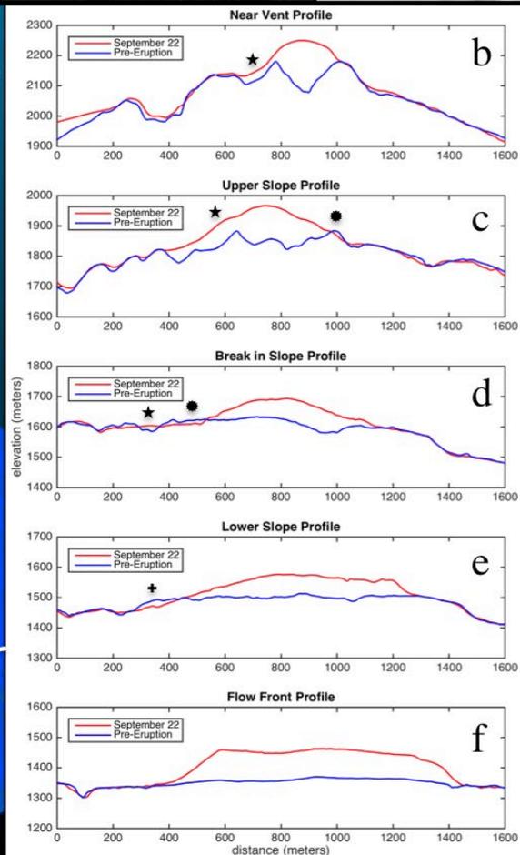
The emplacement of the active lava flow at Sinabung Volcano, Sumatra, Indonesia, documented by structure-from-motion photogrammetry -Carr, et al., 2018. Pre-eruption 5 m DEM and post eruption SfM registered to unchanged areas
