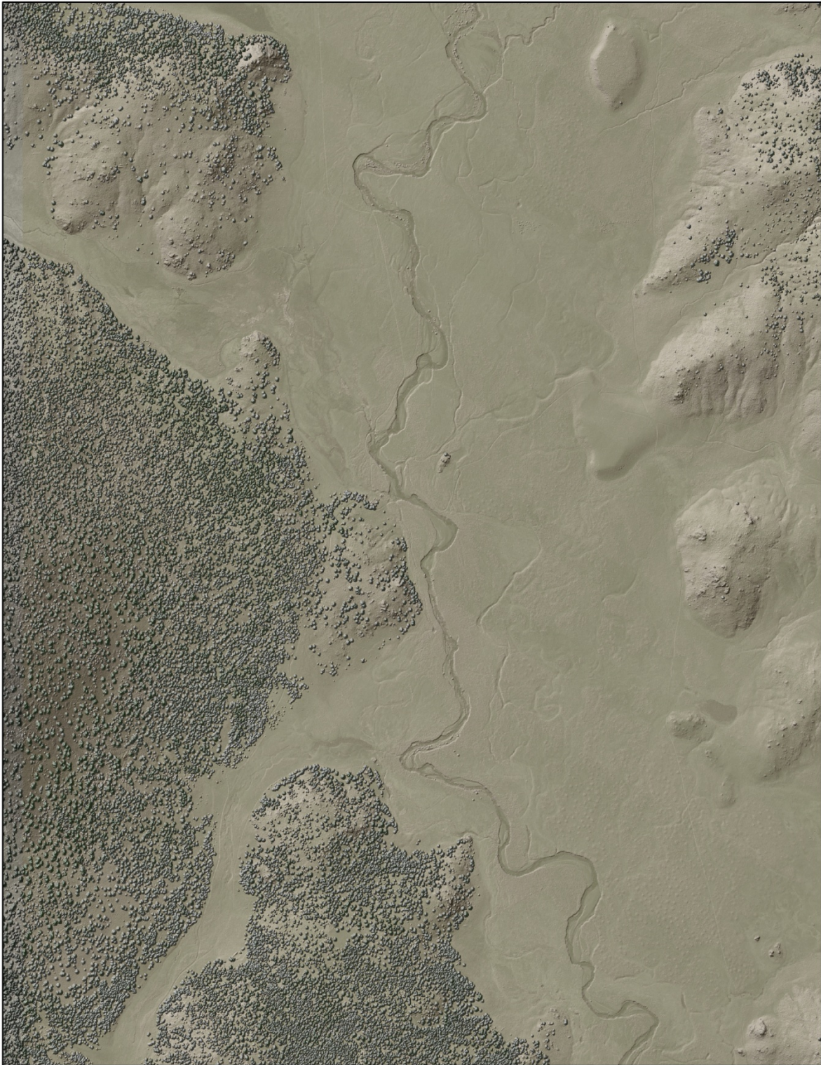
Figure 10. Overhead view of a large meadow in the Kern Plateau survey area. Image created from the highest hit hillshade draped over the intensity TIF and colored by elevation.
