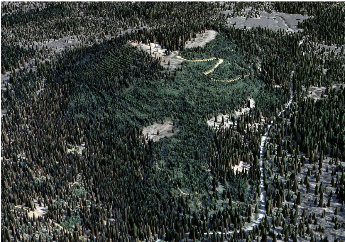
Figure 11: View looking north at Snag Hill in Shasta-Trinity National Forest. Image created from the LiDAR point cloud colored by 2010 NAIP imagery.
