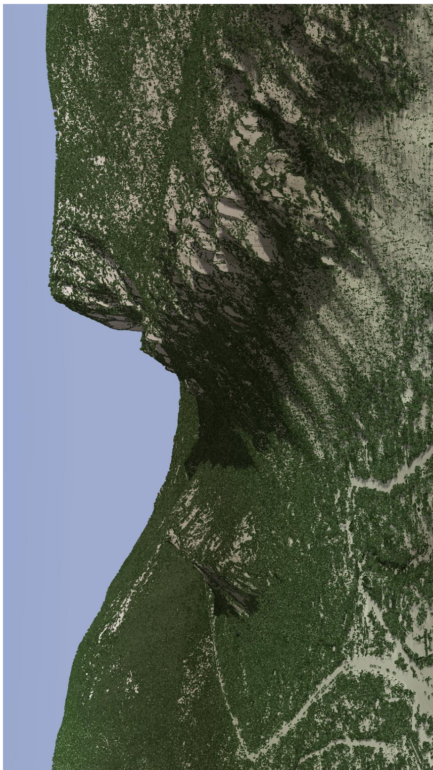
Figure 15: View looking east over the Freds Fire AOI. This image was created from the gridded bare earth model colored by elevation, and overlaid with the above-ground LiDAR point cloud
