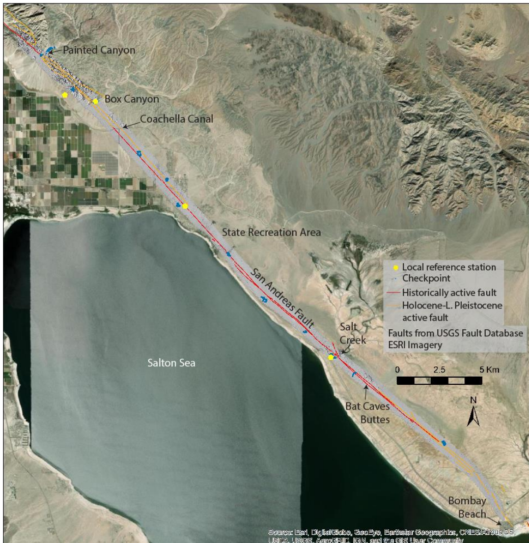
Figure 2. Map showing coverage of our sUAS topographic data set in gray, and locations of our local GNSS reference stations (yellow) and measured checkpoints (blue). Latest Pleistocene to historically active faults from the US Geological Survey Quaternary Fault and Fold Database for reference; ESRI background imagery.
