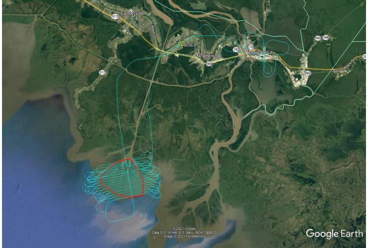
Location of survey polygon, aircraft trajectory, and GNSS reference station
