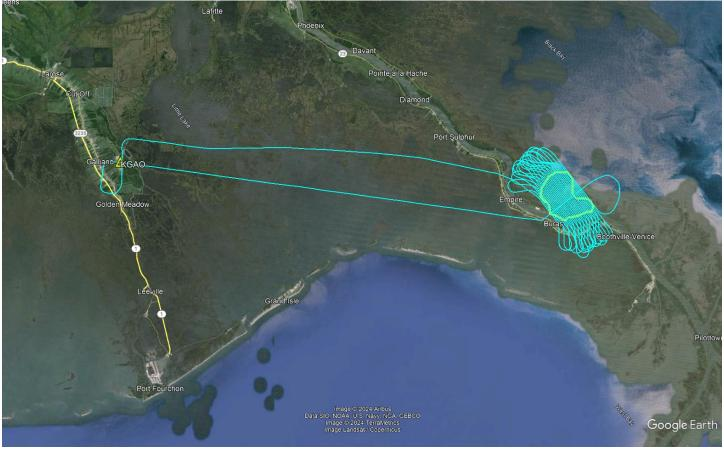
Location of survey polygon, aircraft trajectory, and GNSS reference station
