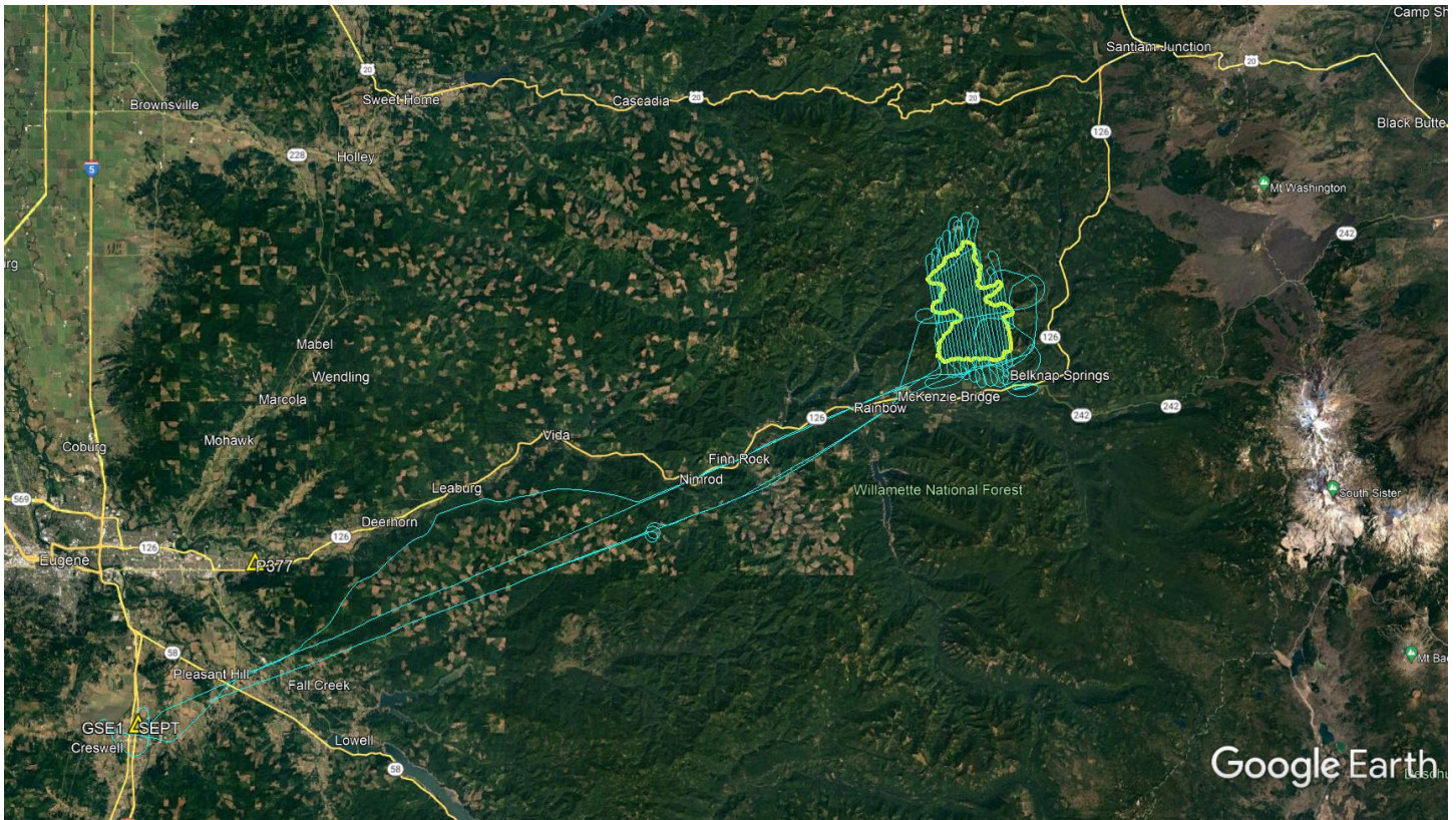
Location of survey polygon, aircraft trajectories, and GNSS reference stations
